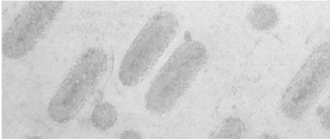
Fig. 2.2.4 TEM image of recorded mark on TDK's BD-R disc
